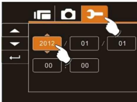
2. Press left/right to highlight each column. Press Up/Down or touch the screen to select the column to adjust the value. Press Menu Button to store the value you change or touch the screen to adjust the Year, Date and Time before pressing the Return Button (
